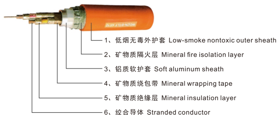
铝护套(柔性)隔离型防火电缆 Aluminum sheathed (flexible) fireproof cable of isolated type
